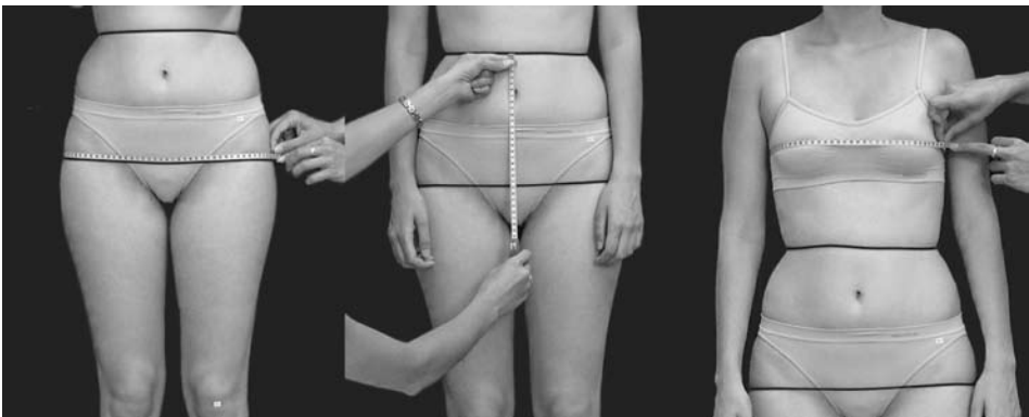
Figure 1: Measurement of the hip girth (left), waist to hip distance (middle) and bust girth (right)
